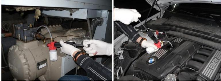
If the knob and the bottleneck are properly tightened, the bottle should fill within seconds. When (almost) full, pull out the tubing from the dipstick's tube or reservoir, unscrew the bottle from the pump and close it. **Do not re-use the tubing.**
