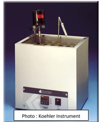
The Copper Corrosion test is a widely used oil analysis method for gearbox, turbine and hydraulic lubricants. This oil analysis method will detect the corrosive effects of a lubricant on copper alloys, but it is ineffective on iron or ferrous alloy parts and components.
